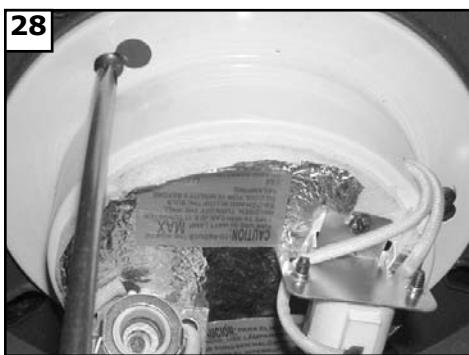
Loosen 3 screws with key slots. Attach fitter by placing over screws and twisting clockwise into place. Tighten all 3 screws securely.
